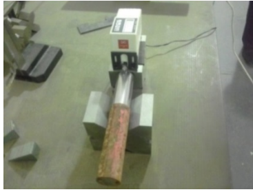
Fig.4 measuring of (SR) by Roughness Tester.
