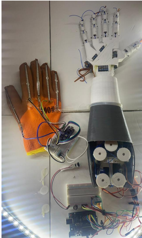
Fig. 10. Robotic hand controlled by glove using Bluetooth
