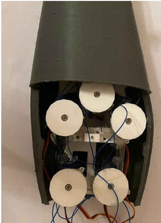
Fig. 8. Arm and servo assembly (made up using 3D printer)
