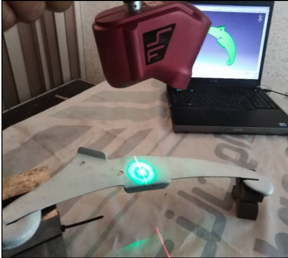
Figure 4. The Baces3D arm during scanning of the sail rib.
