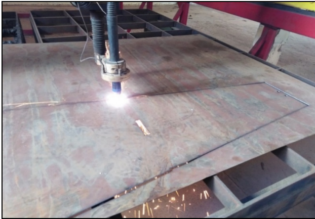
Figure 10. Cutting the Sails using a CNC plasma machine.
