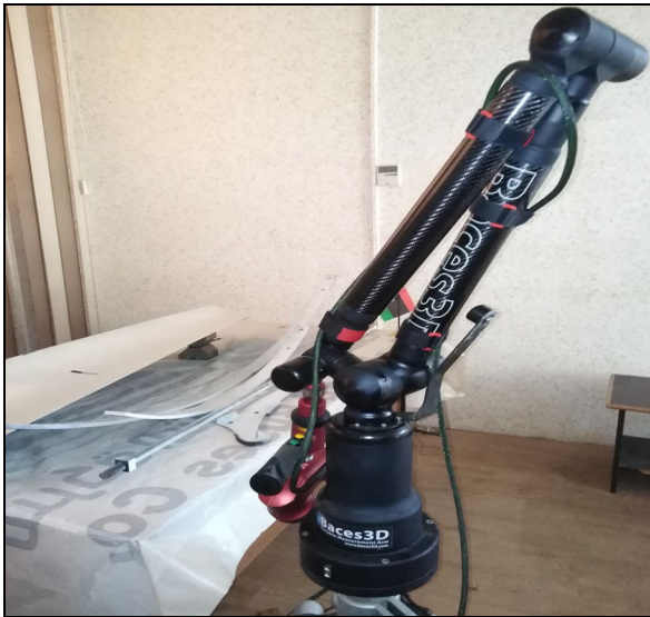
Figure 2. BacesSCAN portable laser scanning system.
