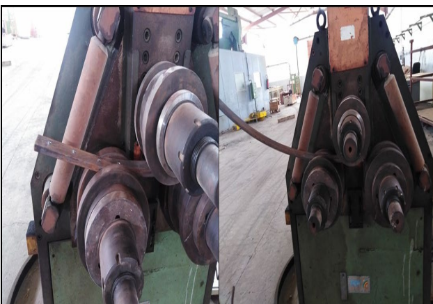
Figure 12. Bending the outer band by CNC rolling machine.
