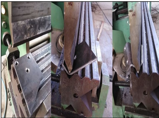
Figure 11. Bending the Sail's tie by the bending press machine.
